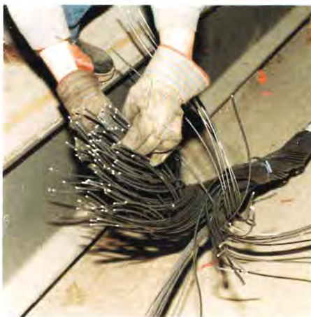
Fig. 12 Conductor AACSR/AC1805/228 after loading to failure
