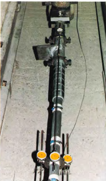
Fig. 21 Testing of the dead-end clamp
