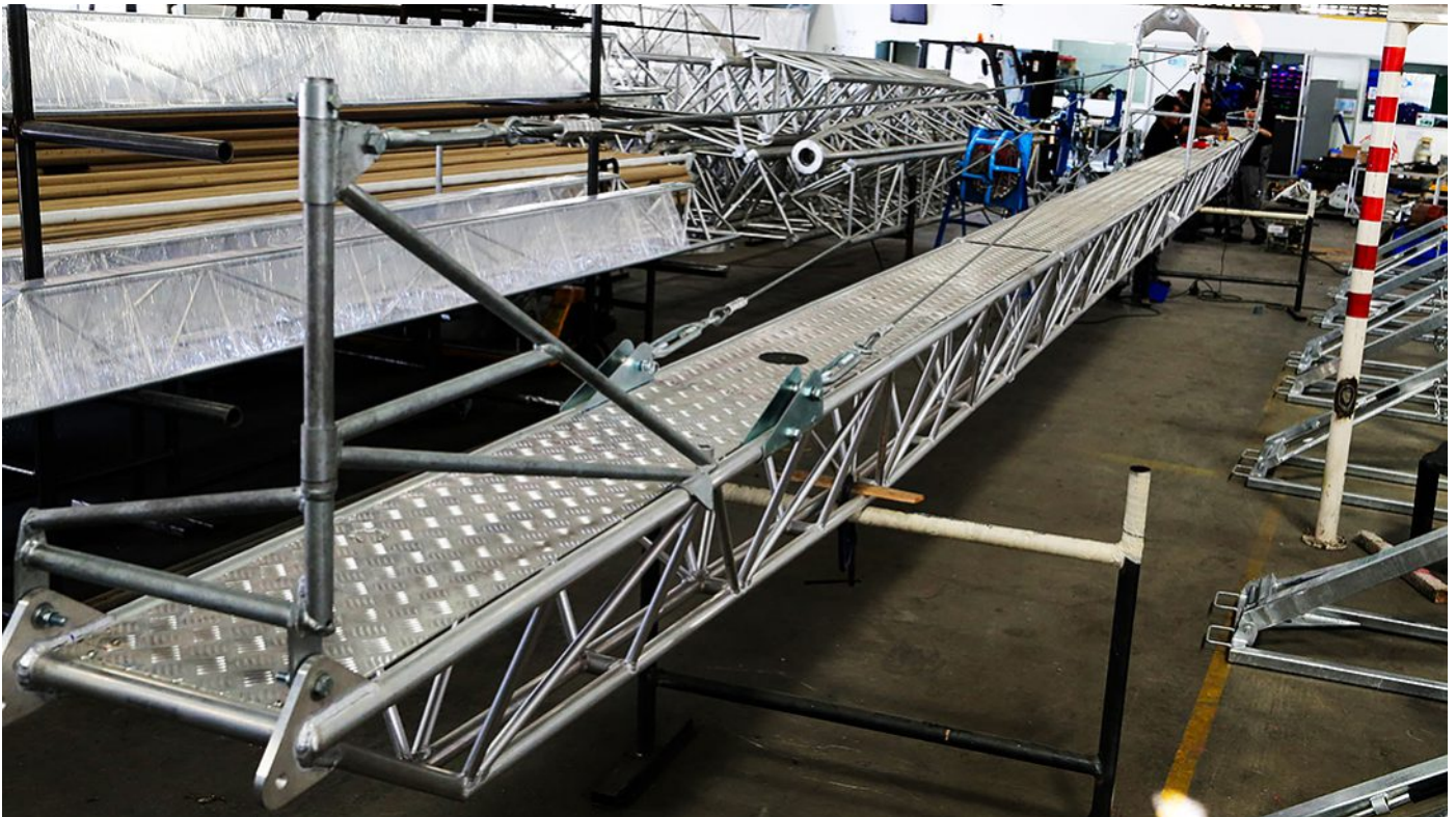
metal sheet coverage on stepping area (PLA-00-0004)
