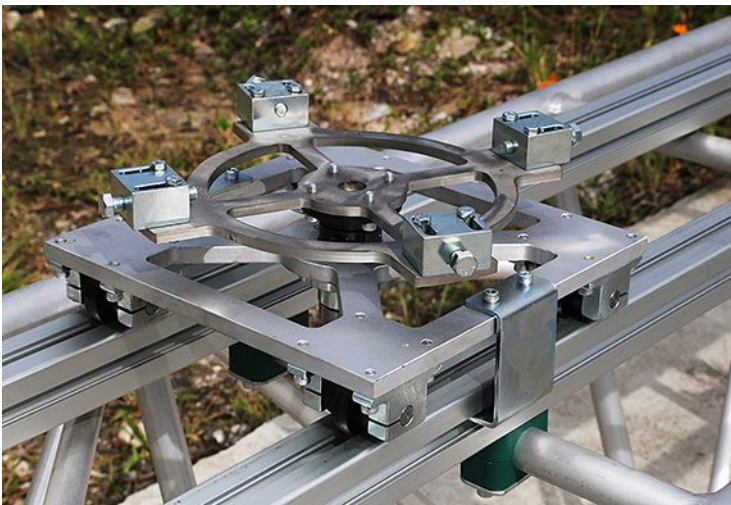
“press trolley PLA-00-0002” on “railway profile PLA-00-0003”
