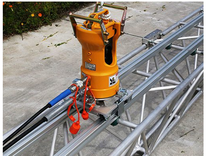
“press trolley PLA-00-0002” on “railway profile PLA-00-0003”
